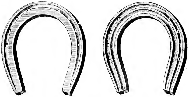
FIG. 126.—FRONT SHOES, MOST SUITABLE FOR RIDING AND CARRIAGE HORSES. 1
